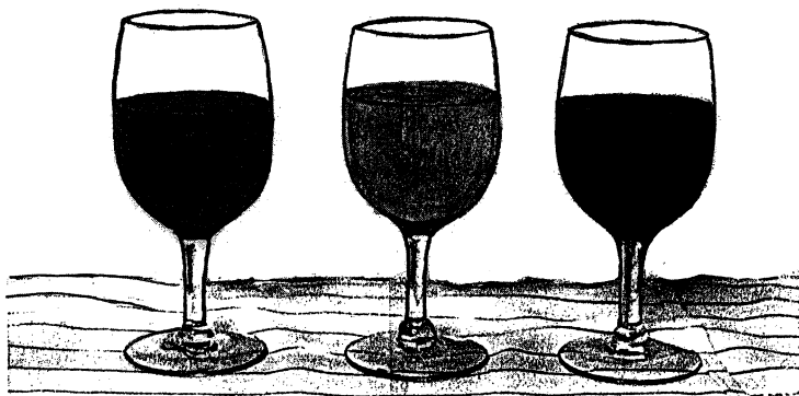
Figure 8. Visible appearance of (left) control hard pressed wine, (middle) ultrafiltered permeate, (right) retentate or rejected wine.
